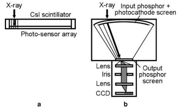
**Figure 2** Components of the detectors: (a) flat panel detector; (b) image intensifier detector
