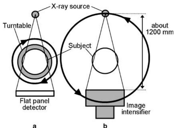
**Figure 1** Experimental set-ups (top view): (a) flat panel detector system; (b) image intensifier detector system
