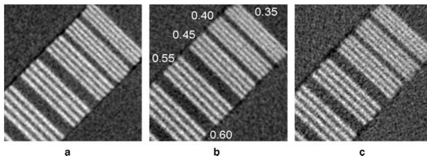
**Figure 5** Three-dimensional images of a high-contrast pattern: (a) coronal image by flat panel detector ( $2 \times 2$ -binning mode); (b) axial image by flat panel detector ( $2 \times 2$ -binning mode); (c) axial image by image intensifier detector ( $4.5''$  mode)
