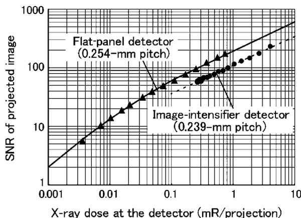
**Figure 4** Signal-to-noise ratio (SNR) of projected images
