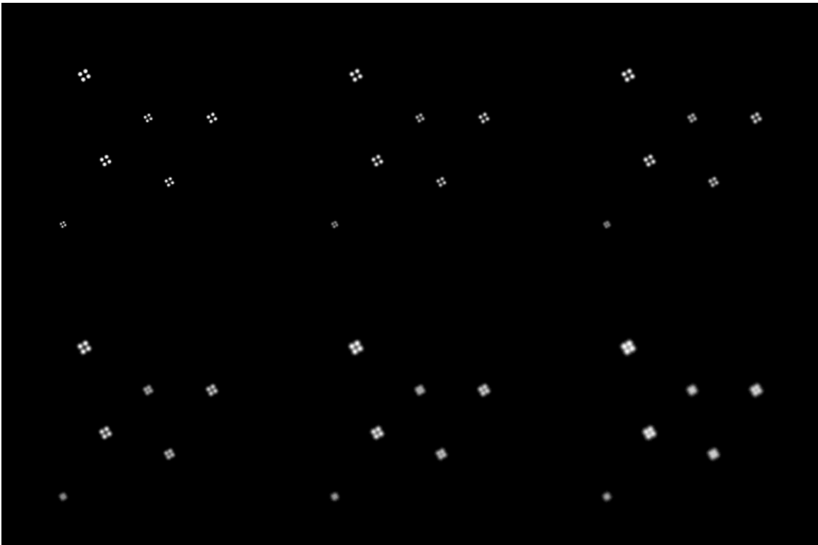
Figure 14. Effect of finite Resolution on the image quality.
